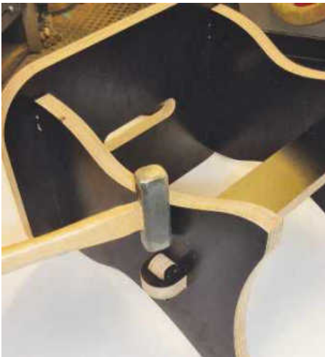
PIC 10. The tenons are tapped into position
